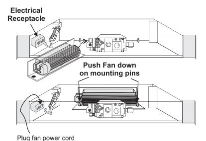
**Optional:** If you require extra space to slide the fan to the back, the left spring can be unhooked from the bracket.
